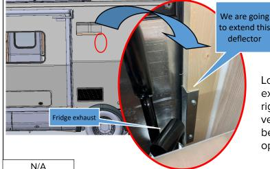
Locate the fridge exhaust at the right side of the vent slightly below the opening
