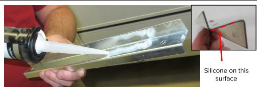
Apply Silicone to the bonding surface of the heat extension.
