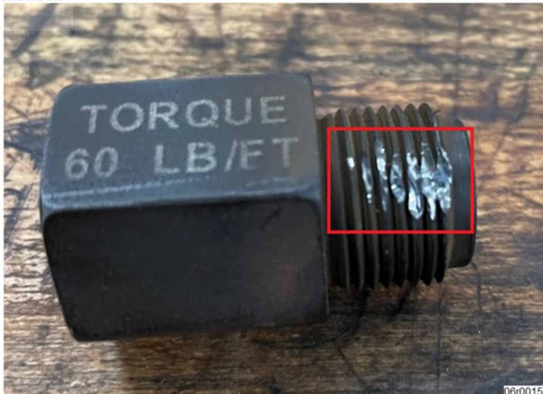
Figure 6, Seal Installer Tool Threads Not Acceptable for Use.
