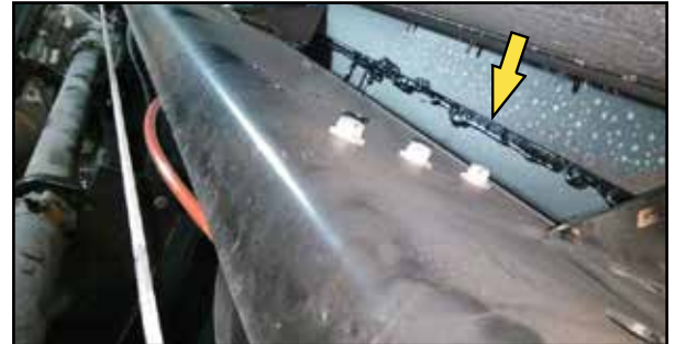
Figure 1-2 Example of how sealant should look
