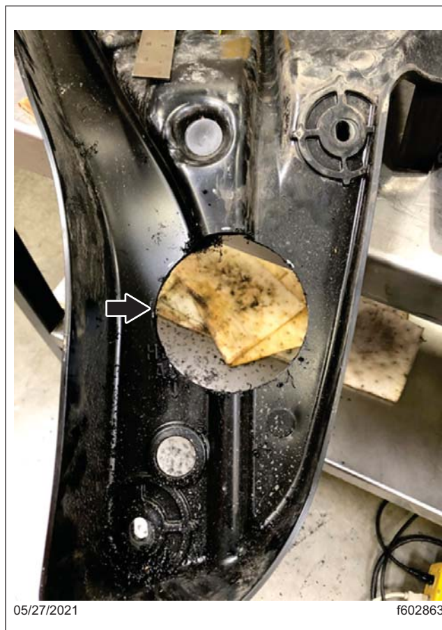
Fig. 4, 4" Hole Drilled in RH Side Hood-Mounted Splash Shield
