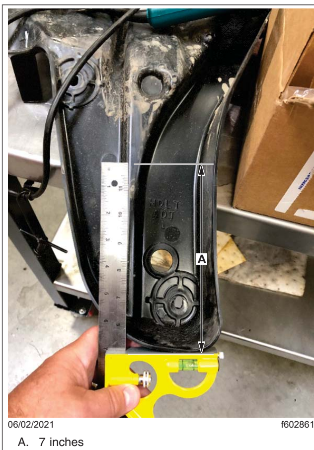
Fig. 2, Using a Machinist's Square for Marking the Center of the Hole
