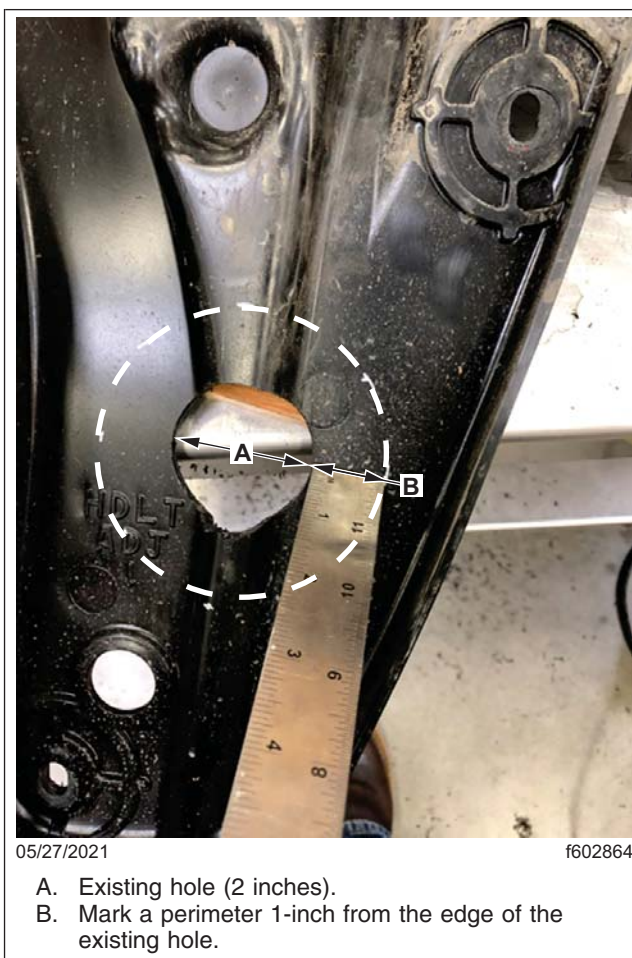
Fig. 5, Marking a 4-Inch Perimeter Concentric to the Existing 2-Inch Hole
