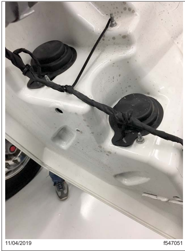
Fig. 12, Lamp Cavity Covers Properly Installed
