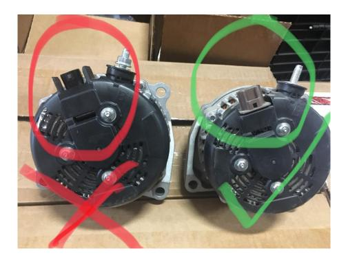
If the cover is found to be **brown**, the regulator is the good one. No further action is required. Replace the splash guard and fill-out the enclosed form accordingly and return it to: <a href="mailto:dealersupport@roadtrekinc.com">dealersupport@roadtrekinc.com</a>
