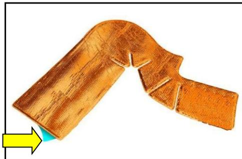
2 C. Apply the heat reflective sheath on the heat guard aiming it as shown in the figure.
