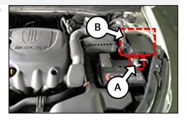
3. Locate the Multi Fuse (C) ESC1 for (QF) Optima or ABS2 for (XMa) Sorento 40A in the fuse box.
