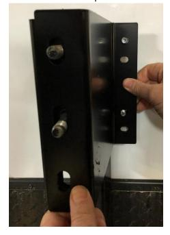
3.) Using just your hand, start threading a 3/8"-16" serrated flange nuts onto 3/8" bolts protruding out of rear wall.
