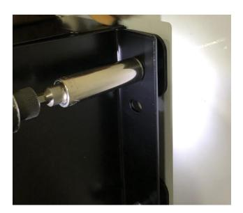
5.) When all 3/8"-16 nuts are tightened, re-check that all nuts are torqued to 30 ft.-lbs. The completed installation should look as shown below.
