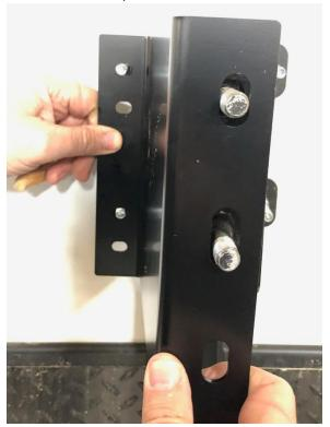
2.) Slide second Z-bracket over spare tire carrier studs and over 3/8" bolts.
