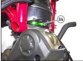
**16.** Protect the engine with a cloth near the ABS control unit and cover the intake manifolds as shown in the figure to avoid the possible penetration of brake fluid or impurities inside the manifolds.
