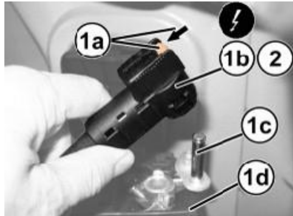
Figure 3 – Battery Negative Cable
