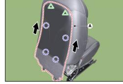
2. Loosen the seat covers on both LH and RH front seats by removing the J-clips and detaching the Velcro as shown in the photos.
