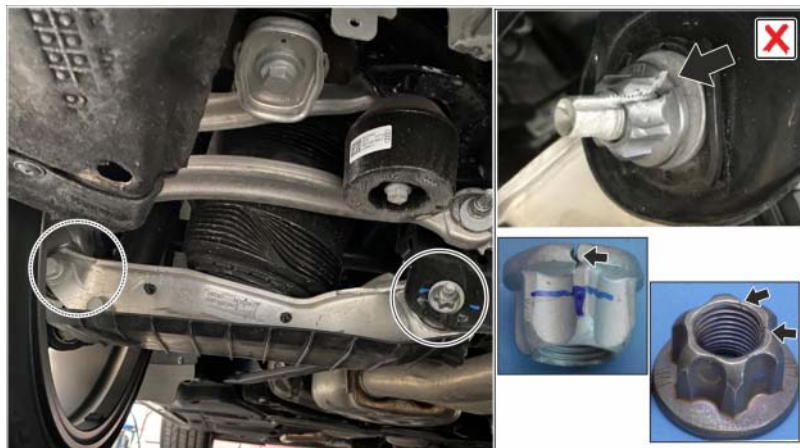
Stress cracks on clamping nuts
