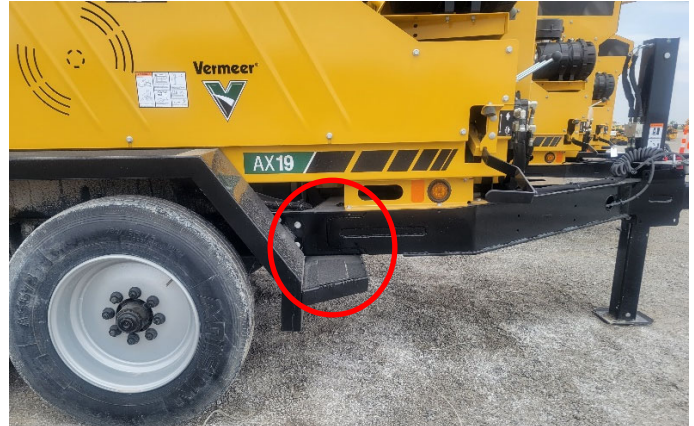
Photo 4 Potential crack location – right side
