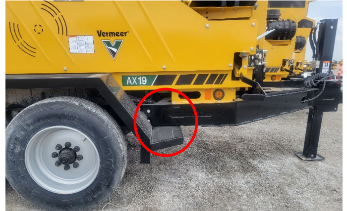
Photo 4 Potential crack location – right side
