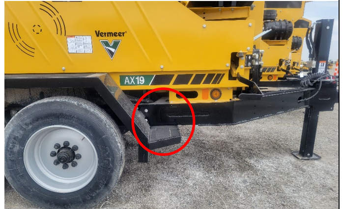
Photo 4 Potential crack location – right side
