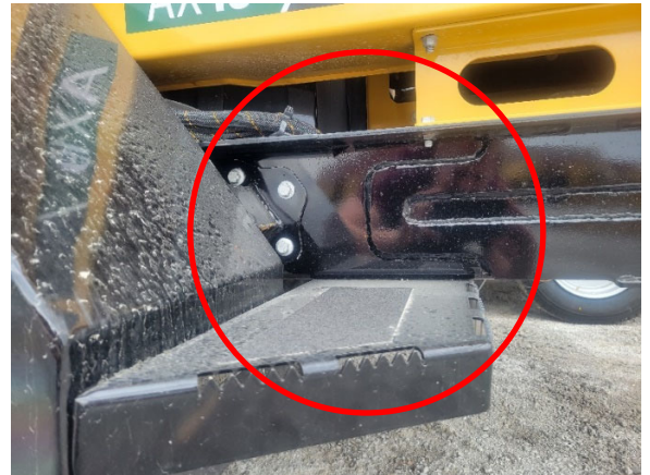
Photo 6 Crack example: frame vertical center
