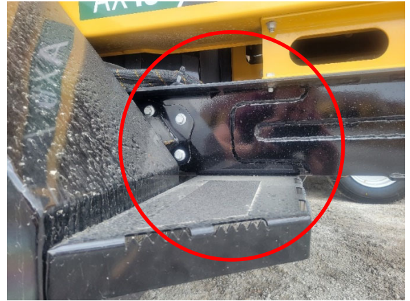
Photo 6 Crack example: frame vertical center
