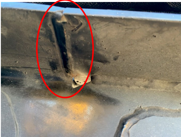
Photo 5 Crack example: frame horizontal top
