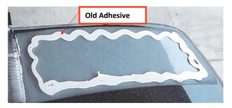
6. Once all the adhesive has been removed, clean the surface of the roof using a hand towel and Isopropyl Alcohol 75%.
