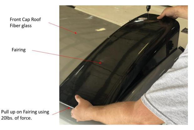
3. If the fairing does not lift up, the fairing is properly secured and no further action is required. If the fairing starts to lift away from the fiberglass, continue to step 4.
