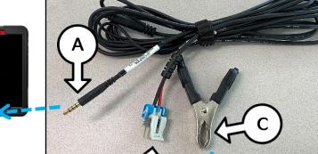
2b. Connect the knocking sensing connector (B) of engine vibration inspection harness to the knock sensor connector on the vehicle.
