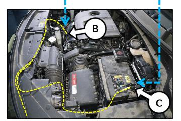
Connect the VCI to the vehicle's OBD2 port and confirm the Bluetooth pairing condition between KDS and VCI.
