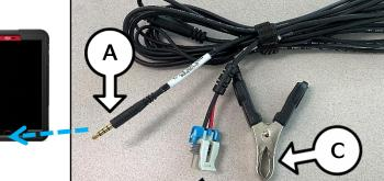
2b. Connect the knocking sensing connector (B) of engine vibration inspection harness to the knock sensor connector on the vehicle.
