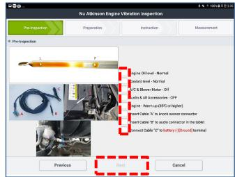
7. The program will automatically check the engine sensor data.
