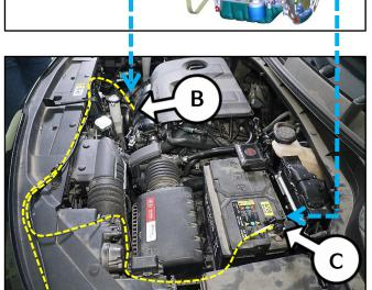
Connect the VCI to the vehicle's OBD2 port and confirm the Bluetooth pairing condition between KDS and VCI.
