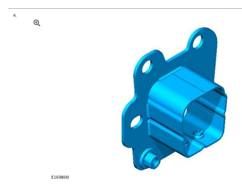
Carefully separate the joints and remove and discard the rear bumper mounting.
