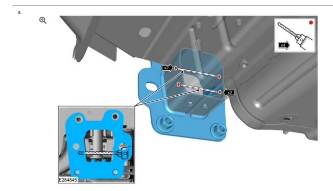
Remove the 4 spot welds shown highlighted in the illustration.
