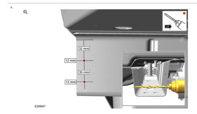
Drill 4, 10 mm holes through both sides of the rear side member in the positions shown in the illustration.
