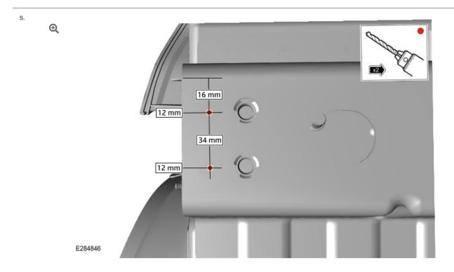
Drill 2, 10 mm holes through the bottom of the rear side rail in the positions shown in the illustration.
