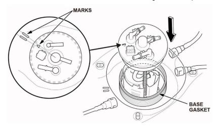
47. Hold the fuel tank unit vertically, and tighten the new fuel tank unit locknut with a new locknut plate by hand.
