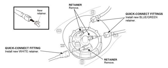
51. Connect the quick-connect fittings to the fuel tank unit.
