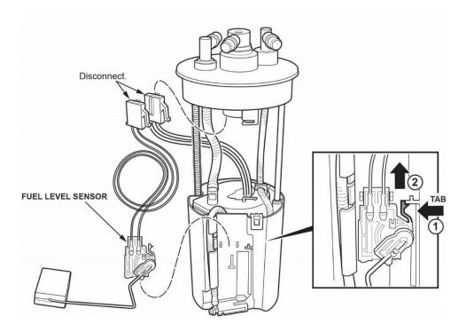
30. Remove the fuel level sensor from the fuel tank unit.
