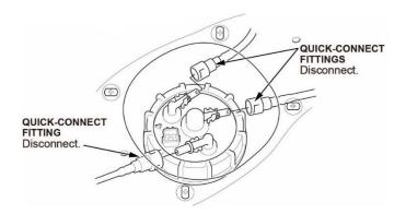
25. Loosen the fuel tank unit locknut using the Fuel Sender Wrench (T/N 07AAA-S0XA100).
