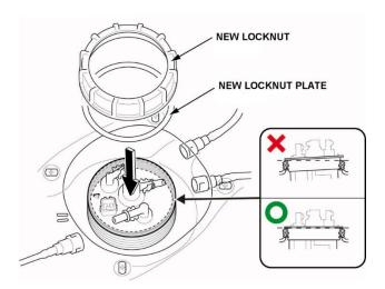
48. Tighten the fuel tank unit locknut to the specified torque using the fuel sender wrench.
