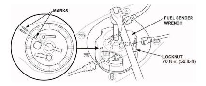
49. If the marks do not line up, friction between the fuel tank unit and the locknut may cause the fuel tank unit to turn while tightening. Observe the difference (shaded area), and loosen the locknut until the fuel tank unit can be rotated. Rotate the fuel tank unit counter-clockwise by the same amount, and repeat the tightening process.
