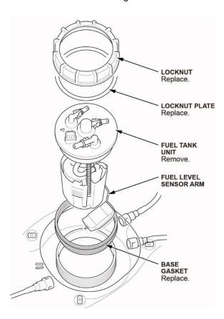
27. Prepare the fuel tank unit and parts to be replaced.
