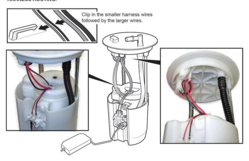
34. While compressing the fuel tank unit, make sure the movement is smooth and the fuel tube and wiring harness do not stretch, pinch, or bind.
