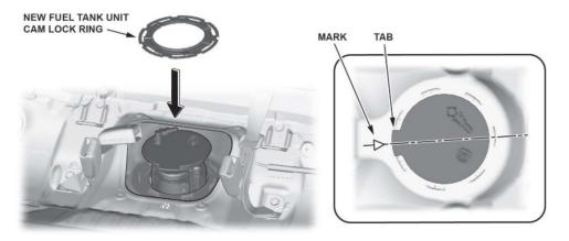
37. Tighten the fuel tank unit cam lock ring.
