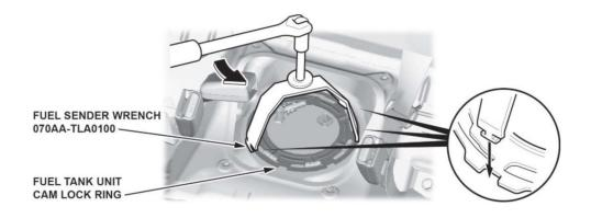
18. Turn the fuel tank unit cam lock ring counterclockwise to unlock it.
