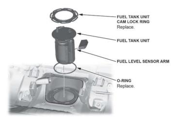
20. Prepare the fuel pump and parts to be replaced.
