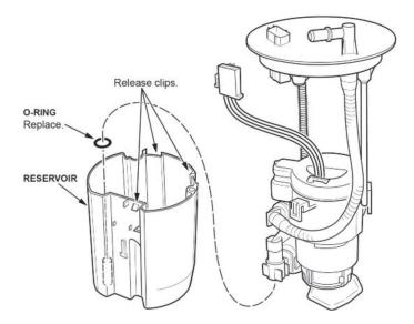
25. Remove the fuel filter assembly from the reservoir by releasing the three clips.
