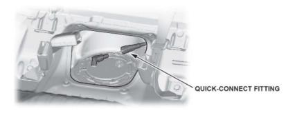
42. Connect the fuel tank unit connector.
