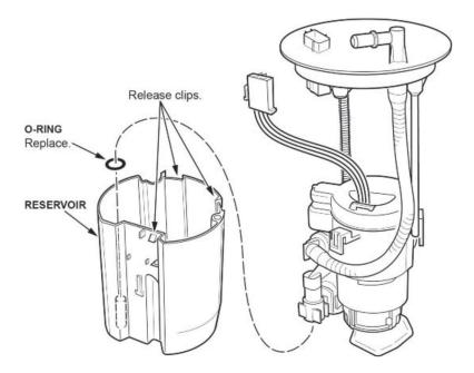
26. Release the three clips at the base of the fuel pump assembly and remove it from the fuel filter.
