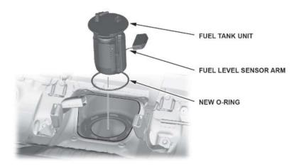
36. Line up the tab of the fuel tank unit as shown, and partially install the new fuel tank unit cam lock ring.
