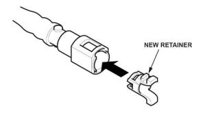
41. Connect the fuel line quick-connect fitting.
