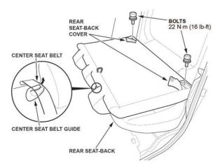
11. Pull out the center seat belt through the slit in the center seat belt guide.
