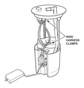
22. Press the tab on the fuel level sensor to release the lock. Then, push up on the fuel level sensor.
