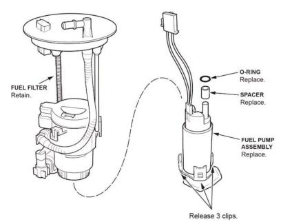
27. Pull the fuel pump assembly out of the fuel filter.
