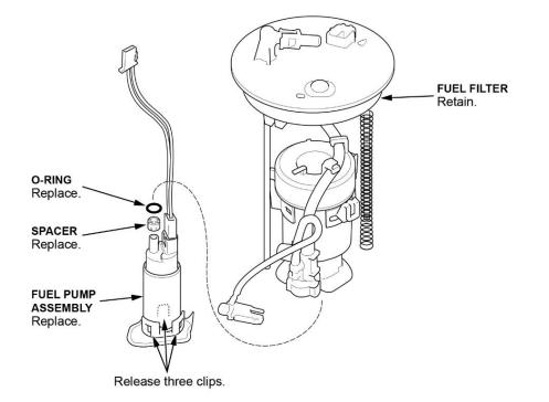
28. Pull the fuel pump assembly out of the fuel filter.
