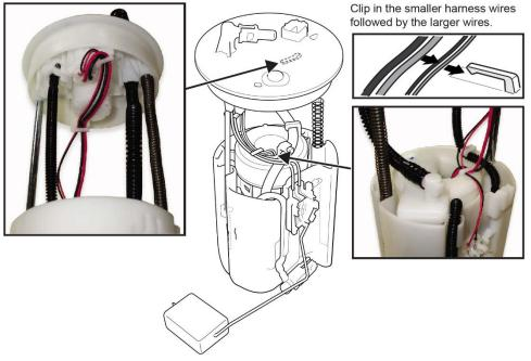
37. While compressing the fuel tank unit, make sure the movement is smooth and the fuel tube and wiring harness do not stretch, pinch, or bind.
