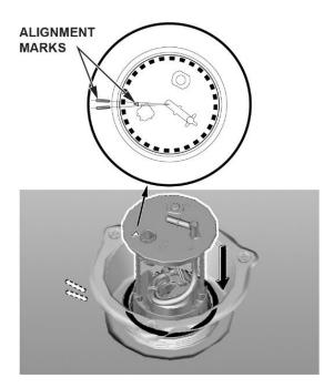
40. Align the mark on the new locknut to the start of the thread on the fuel tank.
