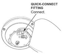
46. Connect the fuel tank unit connector.
