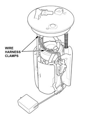
23. Press the tab on the fuel level sensor to release the lock. Then, push up on the fuel level sensor.
