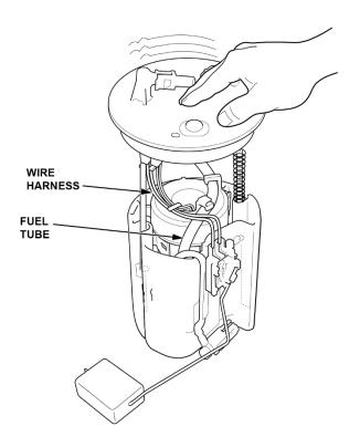
38. Insert the fuel tank unit partially into the fuel tank with a new O-ring.
