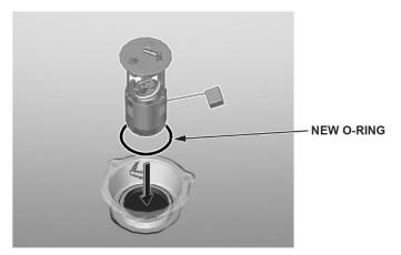
39. Line up the mark on the fuel tank unit to the marks on the fuel tank, then insert the fuel tank unit into the fuel tank. NOTE: To avoid any leaks, check the O-ring, either visually or by hand, to make sure it is not pinched.
