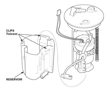
27. Release the three clips at the base of the fuel pump assembly and remove it from the fuel filter.
