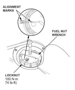
43. *If the marks do not line up*, friction between the fuel tank unit and the locknut may cause the fuel tank unit to turn while tightening. Observe the difference (shaded area), and loosen the locknut until the fuel tank unit can be rotated. Rotate the fuel tank unit **counter-clockwise** by the same amount, and repeat the tightening process.
