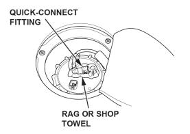
18. Disconnect the quick-connect fitting from the fuel tank unit.
