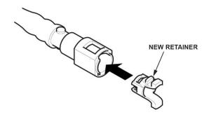
45. Connect the fuel line quick-connect fitting.
