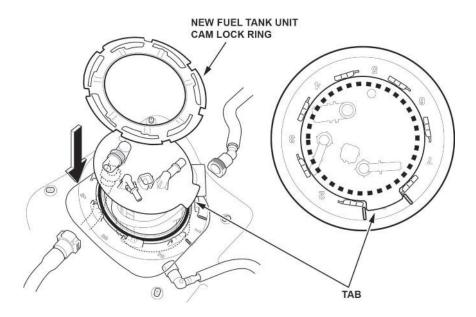
58. Connect the fuel vent tube and fuel tank vapor recirculation tube by slightly turning the fuel tank unit counterclockwise.
