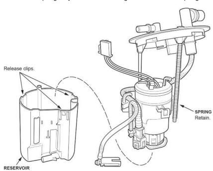
42. Release the three clips at the base of the fuel pump assembly and remove it from the fuel filter.
