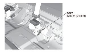
18. Remove the fuel tank unit access panel, and disconnect the connector.
