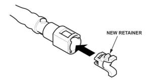
61. Connect the fuel line quick-connect fitting and connector. NOTE: Install the connector cover if it was removed.
