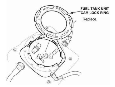
28. Remove the fuel tank unit.
