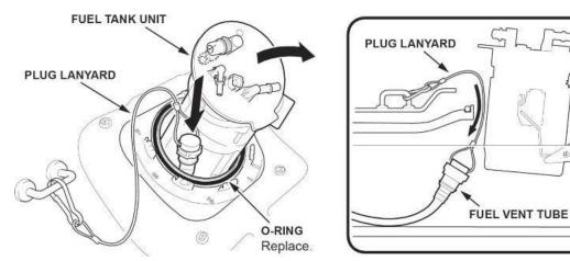
NOTE: It is OK for the plugged tube to be submerged in the fuel.
