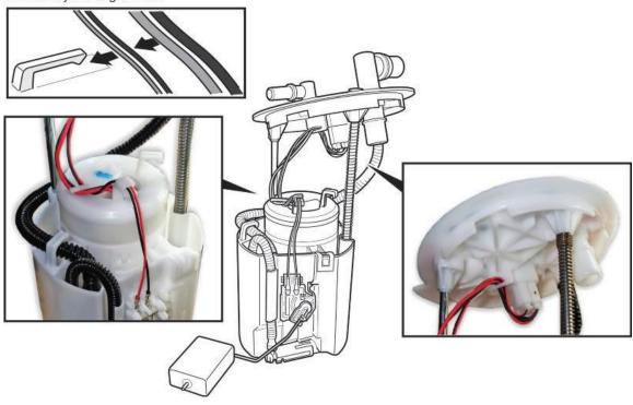
50. While compressing the fuel tank unit, make sure the movement is smooth and the fuel tube and wiring harness do not stretch, pinch or bind.
