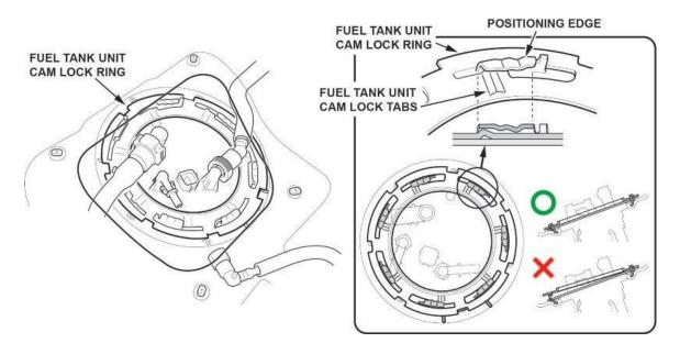
59. Tighten the fuel tank unit cam lock ring by turning clockwise using the fuel sender wrench.
