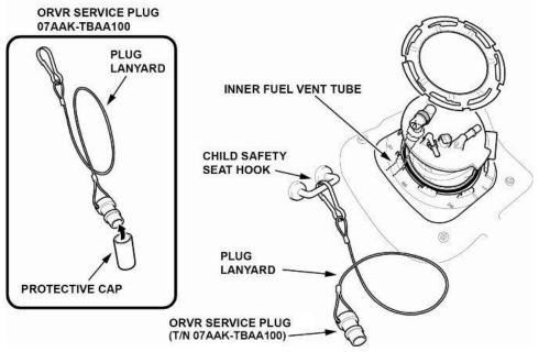
30. Disconnect the inner fuel vent tube from the fuel tank unit, and hold it.
