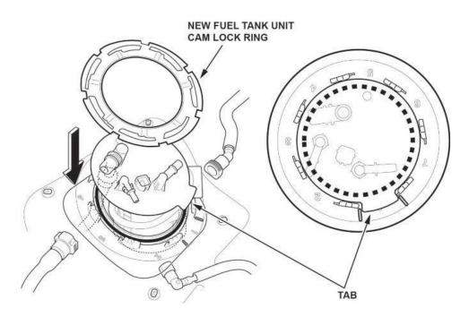
57. Connect the fuel vent tube and fuel tank vapor recirculation tube by slightly turning the fuel tank unit counterclockwise. NOTE: Do not bend the fuel vent tube and fuel tank vapor recirculation tube excessively.
