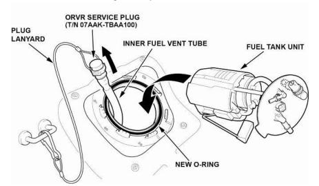
52. Grab the plug lanyard, and pull the inner fuel vent tube up until it is close to the fuel tank opening. Hold the tube while installing the fuel tank unit.
