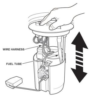
37. Install the fuel tank unit into the fuel tank with a new O-ring.
