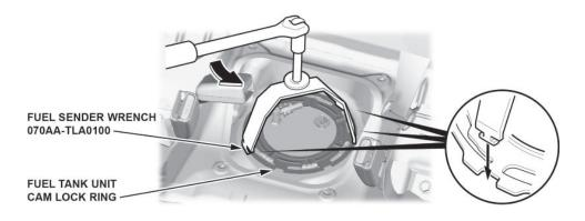
18. Turn the fuel tank unit cam lock ring counterclockwise to unlock it.
