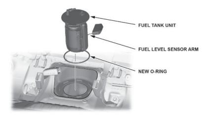
38. Line up the tab of the fuel tank unit as shown, and partially install the new fuel tank unit cam lock ring.
