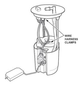
22. Press the tab on the fuel level sensor to release the lock. Then, push up on the fuel level sensor.
