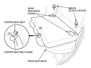
11. Pull out the center seat belt through the slit in the center seat belt guide.
