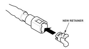
43. Connect the fuel line quick-connect fitting.
