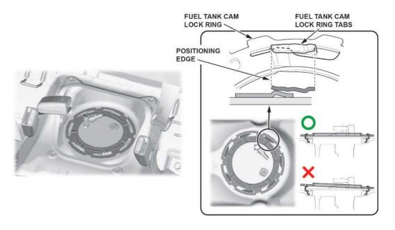
40. Turn the fuel tank unit cam lock ring by hand, and slide the fuel tank unit cam lock tabs to the positioning edge as shown.
