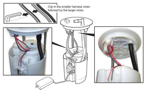
36. While compressing the fuel tank unit, make sure the movement is smooth and the fuel tube and wiring harness do not stretch, pinch, or bind.
