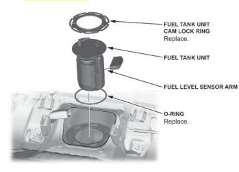
20. Prepare the fuel pump and parts to be replaced.
