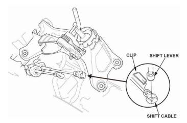
• Disconnect the shift cable from the shift lever.
