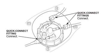
50. Connect the fuel tank unit connector.
