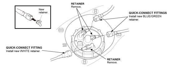
49. Connect the quick-connect fittings to the fuel tank unit.
