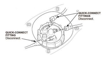
25. Loosen the fuel tank unit locknut using the Fuel Sender Wrench (T/N 07AAA-S0XA100).
