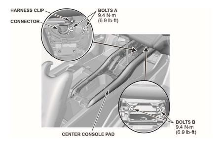
14. Remove the center console pad, and disengage the brackets from the bolts.
