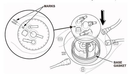
45. Hold the fuel tank unit vertically, and tighten the new fuel tank unit locknut with a new locknut plate by hand.
