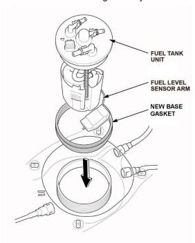
44. Line up the marks on the fuel tank and fuel tank unit as shown, then insert the fuel tank unit.
