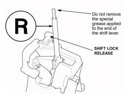
• Insert a 6 mm (0.236 in) pin with no burrs into the positioning holes.
