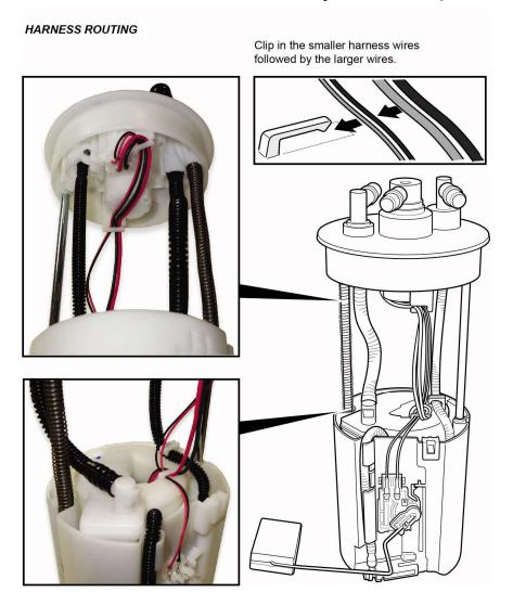
42. While compressing the fuel tank unit, make sure the movement is smooth and the fuel tube and wiring harness do not stretch, pinch, or bind.
