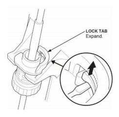
Rotate the socket holder retainer counterclockwise until it stops, then remove the shift cable.
