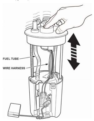
43. Partially insert the fuel tank unit into the fuel tank with a new base gasket.
