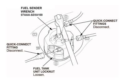
26. Remove the fuel tank unit locknut, then remove the fuel tank unit.
