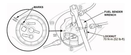
47. If the marks do not line up, friction between the fuel tank unit and the locknut may cause the fuel tank unit to turn while tightening. Observe the difference (shaded area), and loosen the locknut until the fuel tank unit can be rotated. Rotate the fuel tank unit counter-clockwise by the same amount, and repeat the tightening process.
