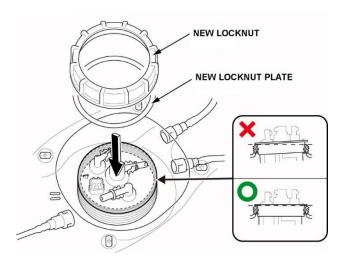
46. Tighten the fuel tank unit locknut to the specified torque using the fuel sender wrench.
