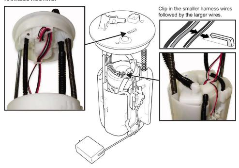
35. While compressing the fuel tank unit, make sure the movement is smooth and the fuel tube and wiring harness do not stretch, pinch, or bind.
