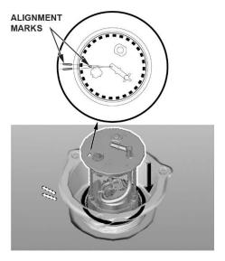
38. Line up the mark on the new locknut to the start of the thread on the fuel tank.
