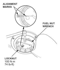
41. If the marks do not line up, friction between the fuel tank unit and the locknut may cause the fuel tank unit to turn while tightening. Observe the difference (shaded area), and loosen the locknut until the fuel tank unit can be rotated. Rotate the fuel tank unit counter-clockwise by the same amount, and repeat the tightening process.
