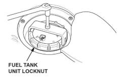
20. Remove the fuel tank unit locknut, then remove the fuel tank unit.
