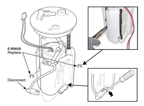
25. Disconnect the joint at the bottom of the reservoir.
