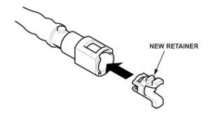
43. Connect the fuel line quick-connect fitting.
