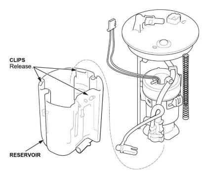
27. Release the three clips at the base of the fuel pump assembly and remove it from the fuel filter.
