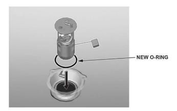
37. Line up the mark on the fuel tank unit to the marks on the fuel tank, then insert the fuel tank unit into the fuel tank. NOTE: To avoid any leaks, check the O-ring, either visually or by hand, to make sure it is not pinched.
