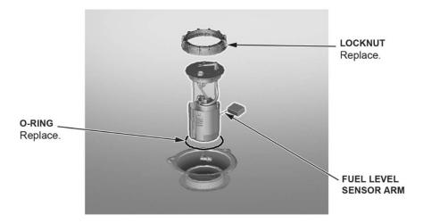
21. Prepare the fuel tank unit and parts to be replaced.
