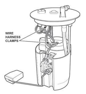
22. Press the tab on the fuel level sensor to release the lock. Then, push up on the fuel level sensor.
