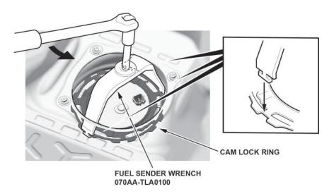
18. Turn the fuel tank unit cam lock ring counterclockwise to unlock it.
