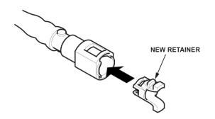
41. Connect the fuel line quick-connect fitting.
