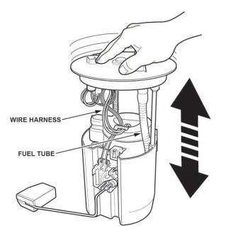
37. Line up the tab of the fuel tank unit as shown, and partially install the new fuel tank unit cam lock ring with a new O-ring.
