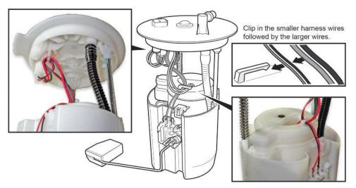
36. While compressing the fuel tank unit, make sure the movement is smooth and the fuel tube and wiring harness do not stretch, pinch, or bind.
