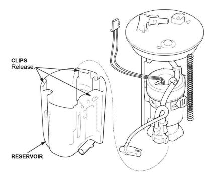
30. Release the three clips at the base of the fuel pump assembly and remove it from the fuel filter.
