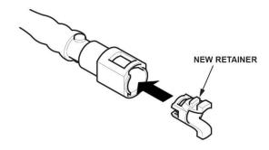
45. Connect the fuel line quick-connect fitting.
