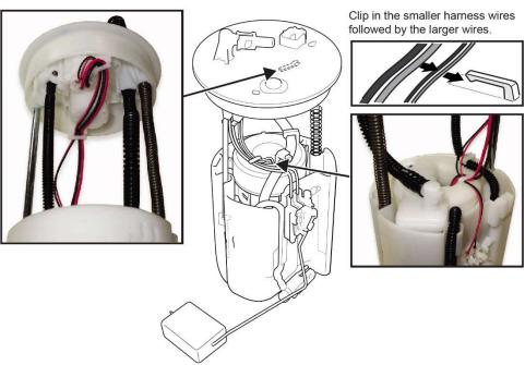
38. While compressing the fuel tank unit, make sure the movement is smooth and the fuel tube and wiring harness do not stretch, pinch, or bind.
