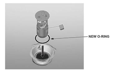
40. Line up the mark on the fuel tank unit to the marks on the fuel tank, then insert the fuel tank unit into the fuel tank. NOTE: To avoid any leaks, check the O-ring, either visually or by hand, to make sure it is not pinched.
