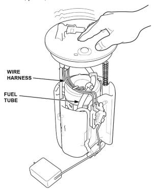
39. Insert the fuel tank unit partially into the fuel tank with a new O-ring.
