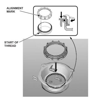
42. Press down on the fuel tank unit while turning the locknut clockwise by hand.
