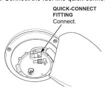
46. Connect the fuel tank unit connector.
