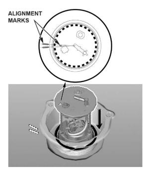
41. Line up the mark on the new locknut to the start of the thread on the fuel tank.
