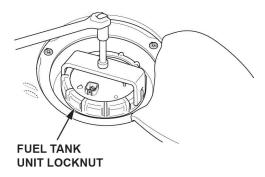
23. Remove the fuel tank unit locknut, then remove the fuel tank unit.
