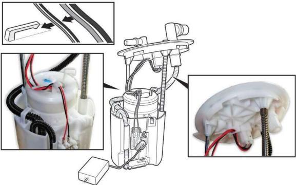
48. While compressing the fuel tank unit, make sure the movement is smooth and the fuel tube and wiring harness do not stretch, pinch, or bind.
