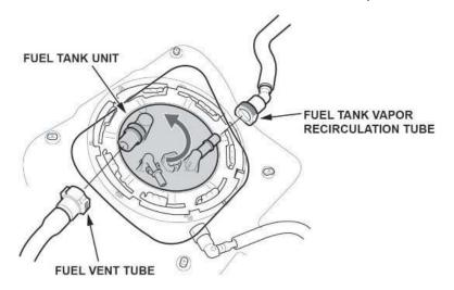
56. Turn the fuel tank unit cam lock ring by hand, and slide the fuel tank unit cam lock tabs to the positioning edge as shown.
