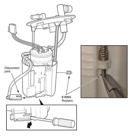
39. Disconnect the joint at the bottom of the reservoir.
