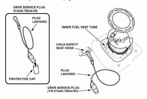
30. Disconnect the inner fuel vent tube from the fuel tank unit, and hold it.
