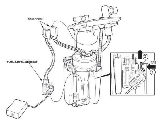
37. Disconnect the fuel level sensor harness and remove the fuel level sensor from the fuel tank unit.
