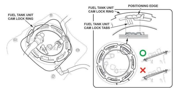
57. Tighten the fuel tank unit cam lock ring by turning clockwise using the fuel sender wrench.
