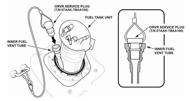
31. Install the ORVR service plug to the inner fuel vent tube. Make sure the ORVR service plug is fully seated by holding the inner fuel vent tube and gently pulling on the plug's lanyard.
