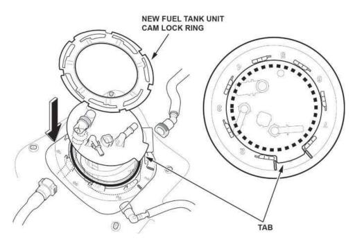
55. Connect the fuel vent tube and fuel tank vapor recirculation tube by slightly turning the fuel tank unit counterclockwise. NOTE: Do not bend the fuel vent tube and fuel tank vapor recirculation tube excessively.
