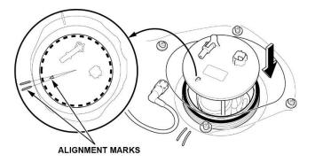
33. Align the mark on the new locknut to the start of the thread on the fuel tank.
