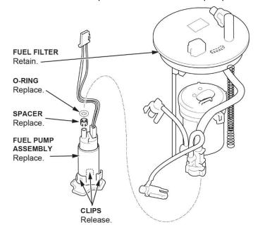
23. Pull the fuel pump assembly out of the fuel filter.
