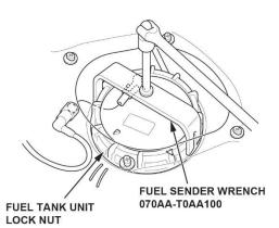
12. Remove the fuel tank unit.
