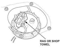
11. Remove the fuel tank unit locknut using the fuel sender wrench (T/N 070AA-T0AA100) as shown. NOTE: Keep the fuel sender wrench from floating.
