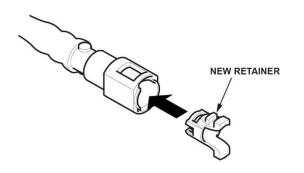
37. Connect the fuel line quick-connect fitting.
