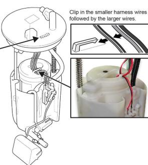
30. While compressing the fuel tank unit, make sure the movement is smooth and the fuel tube and wiring harness do not stretch, pinch, or bind.
