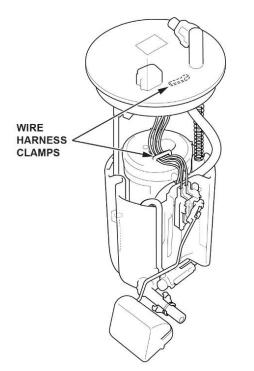
16. Press the tab on the fuel level sensor to release the lock. Then, push up on the fuel level sensor.
