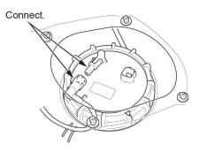
38. Connect the fuel tank unit connector.
