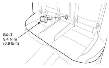
6. While pushing down on the rear seat cushion, pull the seat hook handles to release the hooks. *With rear seat heaters:* Disconnect the connectors and remove the harness clips.
