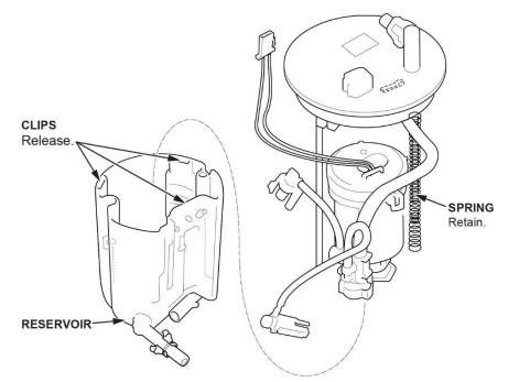
22. Release the three clips at the base of the fuel pump assembly and remove it from the fuel filter.
