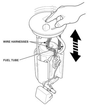
31. Install the new O-ring to the fuel tank, then partially install the new fuel tank unit and connect the transfer pipe quickconnect fitting.
