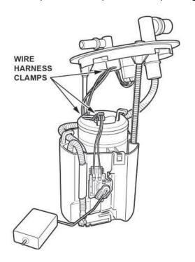
36. Press the tab on the fuel level sensor to release the lock. Then, push up on the fuel level sensor.
