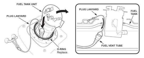
33. Remove the fuel tank unit with the O-ring.
