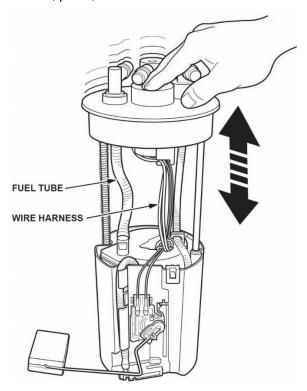
41. Partially insert the fuel tank unit into the fuel tank with a new base gasket.
