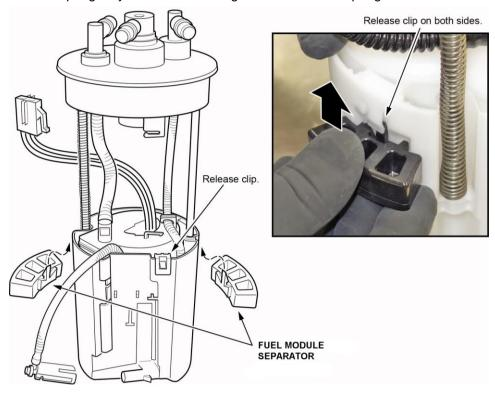
30. Release the three clips at the base of the fuel pump assembly.
