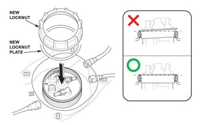
44. Tighten the fuel tank unit locknut to the specified torque using the fuel sender wrench.
