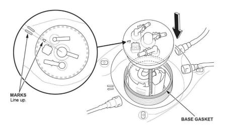
43. Hold the fuel tank unit vertically, and tighten the new fuel tank unit locknut with a new locknut plate by hand.
