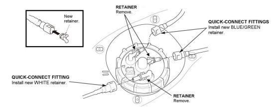
47. Connect the quick-connect fittings to the fuel tank unit.
