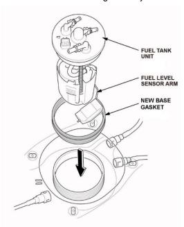
42. Line up the marks on the fuel tank and fuel tank unit as shown, then insert the fuel tank unit.
