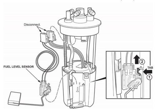
26. Remove the fuel level sensor from the fuel tank unit.
