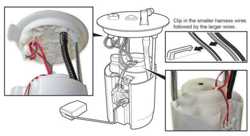
33. While compressing the fuel tank unit, make sure the movement is smooth and the fuel tube and wiring harness do not stretch, pinch, or bind.
