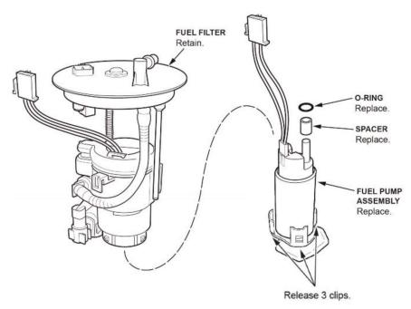
26. Pull the fuel pump assembly out of the fuel filter.
