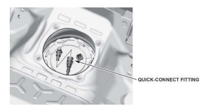
40. Connect the fuel tank unit connector.
