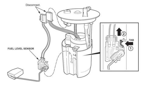
22. Disconnect the fuel level sensor harness, and remove the fuel level sensor from the fuel tank unit.
