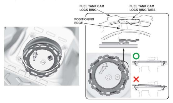
37. Tighten the fuel tank unit cam lock ring by turning clockwise using the fuel sender wrench.
