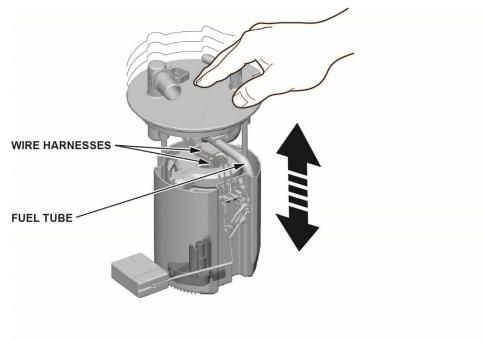
42. Install the fuel tank unit into the fuel tank with a new O-ring.
