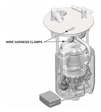
27. Press the tab on the fuel level sensor to release the lock. Then, push up on the fuel level sensor.
