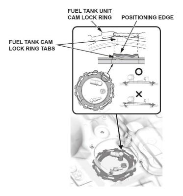
49. Tighten the fuel tank unit cam lock ring by turning clockwise using the fuel sender wrench.
