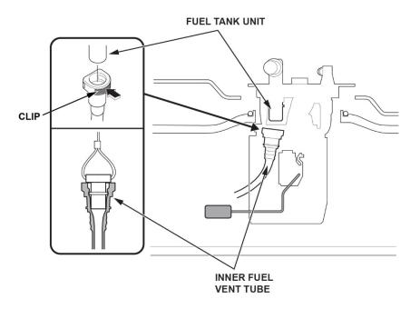
22. Install the ORVR service plug to the inner fuel vent tube. Make sure the ORVR service plug is fully seated by holding the inner fuel vent tube and gently pulling on the plug's lanyard.
