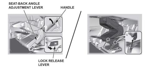
Pull the lock release lever, tilt the seat-back forward and the lift the rear of the seat.
