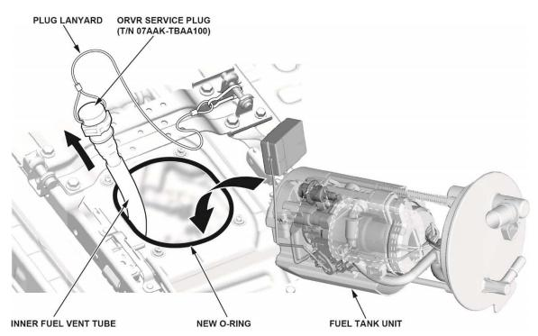
43. Grab the plug lanyard, and pull the inner fuel vent tube up until it is close to the fuel tank opening. Hold the tube while installing the fuel tank unit.
