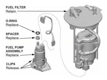
32. Pull the fuel pump assembly out of the fuel filter.
