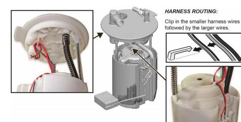
41. While compressing the fuel tank unit, make sure the movement is smooth and the fuel tube and wiring harness do not stretch, pinch, or bind.
