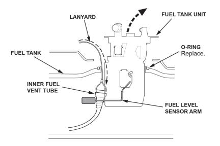
24. Remove the fuel tank unit with the O-ring.
