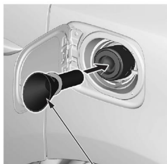
EMERGENCY FUEL FILL FUNNEL
