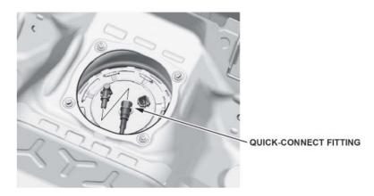
40. Connect the fuel tank unit connector.
