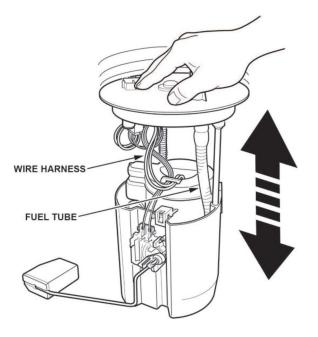
35. Line up the tab of the fuel tank unit as shown, and partially install the new fuel tank unit cam lock ring with a new O-ring.
