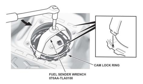
Turn the fuel tank unit cam lock ring counterclockwise to unlock it.
