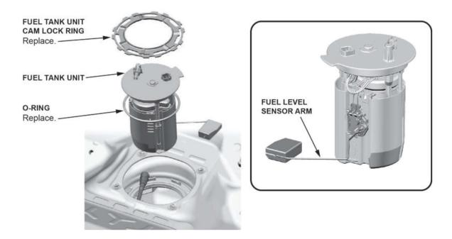
20. Prepare the fuel pump and parts to be replaced.
