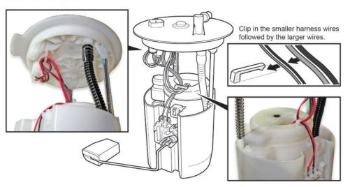
34. While compressing the fuel tank unit, make sure the movement is smooth and the fuel tube and wiring harness do not stretch, pinch, or bind.
