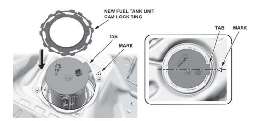
36. Turn the fuel tank unit cam lock ring by hand, and slide the fuel tank unit cam lock tabs to the positioning edge as shown.
