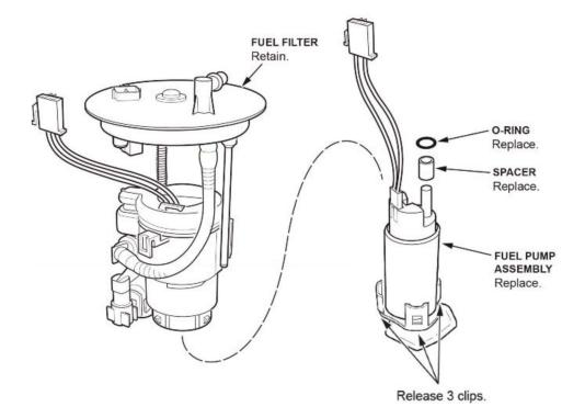
27. Pull the fuel pump assembly out of the fuel filter.
