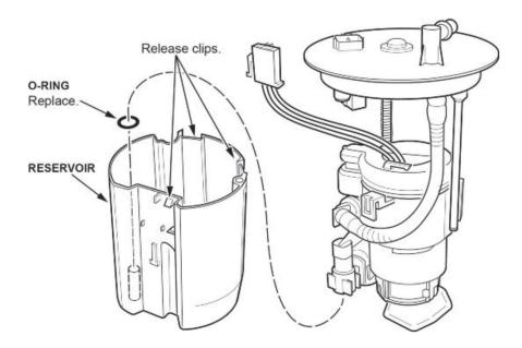
26. Release the three clips at the base of the fuel pump assembly and remove it from the fuel filter.
