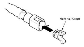
37. Connect the fuel line quick-connect fitting.
