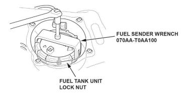
12. Remove the fuel tank unit.
