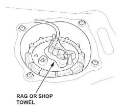
11. Remove the fuel tank unit locknut using the fuel sender wrench (T/N 070AA-T0AA100) as shown.
