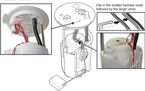
30. While compressing the fuel tank unit, make sure the movement is smooth and the fuel tube and wiring harness do not stretch, pinch, or bind.
