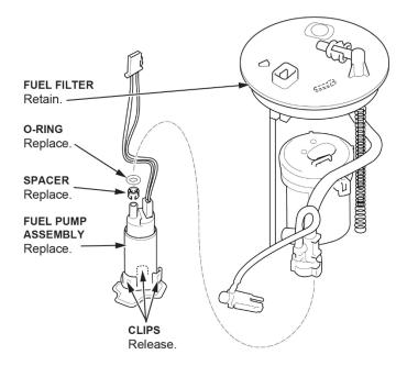
21. Pull the fuel pump assembly out of the fuel filter.
