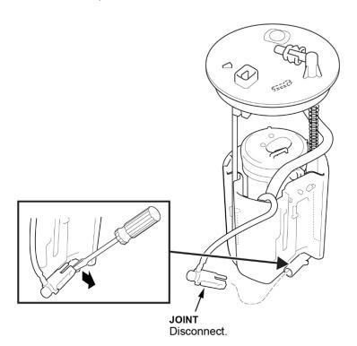
19. Remove the fuel filter assembly from the reservoir by releasing the three clips.
