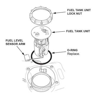
13. Prepare the fuel pump and parts to be replaced.
