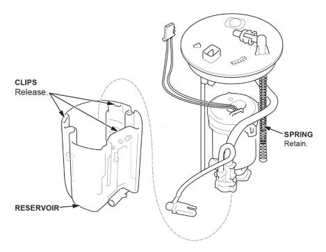
20. Release the three clips at the base of the fuel pump assembly and remove it from the fuel filter.
