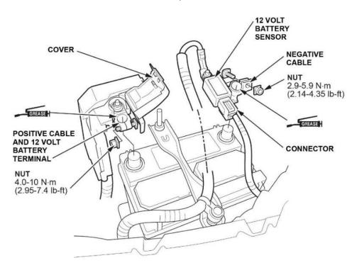
10. Remove the harness clip and connectors as shown.
