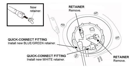
46. Connect the fuel line quick-connect fittings to the fuel tank unit.
