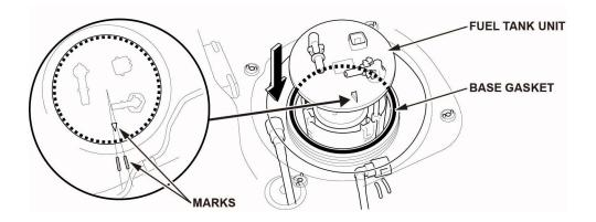
38. While pushing down on the fuel tank unit, make sure the fuel tank unit is flat against the base gasket. To avoid a leak and/or damaging the gasket, make sure the gasket is not pinched. Do this either visually and/or by hand.
