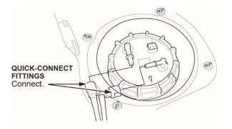
47. Connect the fuel tank unit connector.
