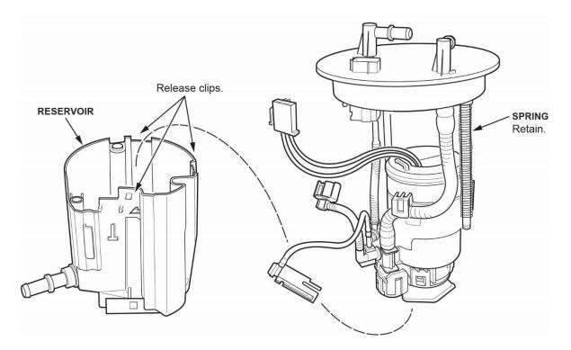
24. Release the three clips at the base of the fuel pump assembly and remove it from the fuel filter.
