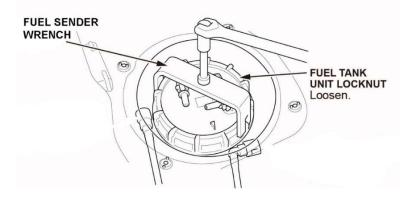
15. Lift the fuel tank unit, and disconnect the transfer tube. Then, remove the fuel tank unit.
