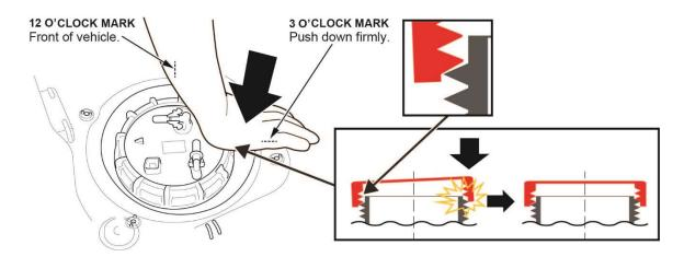
41. Rotate the locknut clockwise 195 degrees from the thread starting point.
