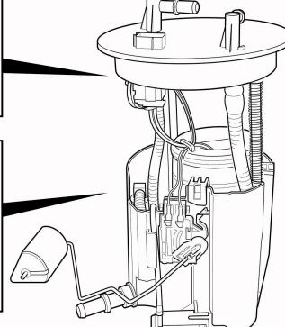
33. While compressing the fuel tank unit, make sure the movement is smooth and the fuel tube and wiring harness do not stretch, pinch, or bind.
