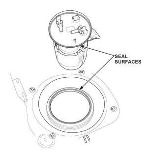
35. Carefully install a new base gasket to the gasket groove on the fuel tank as shown.
