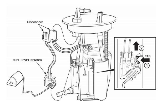
19. Disconnect the fuel level sensor harness and remove the fuel level sensor from the fuel tank unit.
