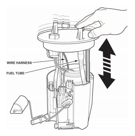
34. Clean the seal surfaces on the fuel tank unit and gasket groove on the fuel tank.
