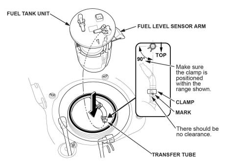
37. Line up the mark on the fuel tank unit to the marks on the fuel tank, then insert the fuel tank unit into the fuel tank. NOTE: To avoid any leaks, check the O-ring, either visually or by hand, to make sure it is not pinched.
