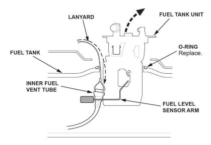
24. Remove the fuel tank unit with the O-ring.
