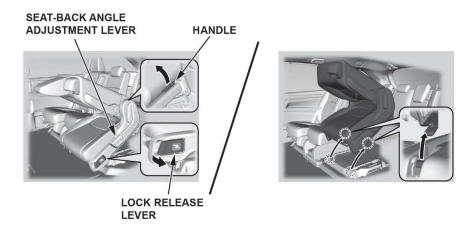
6. Pull the lock release lever, tilt the seat-back forward and the lift the rear of the seat.
