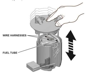
40. Install the fuel tank unit into the fuel tank with a new O-ring.
