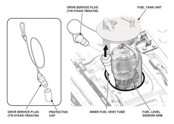
44. Remove the ORVR service plug from the child safety seat hook, and install the provided protective cap.
