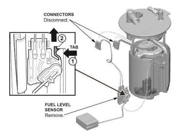
28. Disconnect the fuel level sensor harness, and remove the fuel level sensor from the fuel tank unit.
