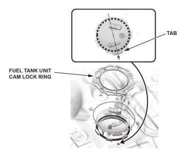
46. Rotate the fuel tank unit cam lock ring (A) and slide the fuel tank unit cam lock tabs (B) into the positioning edge (C) slightly as shown by hand.
