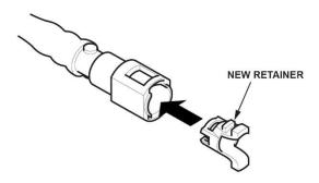
49. Connect the fuel vapor hose, the fuel line quick-connect fitting, and fuel tank unit connector.
