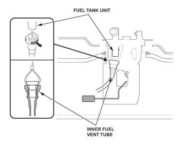
22. Install the ORVR service plug to the inner fuel vent tube. Make sure the ORVR service plug is fully seated by holding the inner fuel vent tube and gently pulling on the plug's lanyard.
