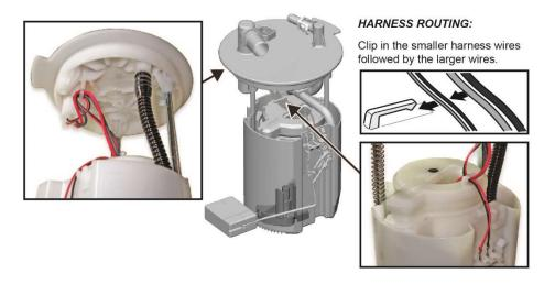
39. While compressing the fuel tank unit, make sure the movement is smooth and the fuel tube and wiring harness do not stretch, pinch, or bind.
