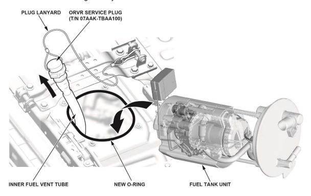
41. Grab the plug lanyard, and pull the inner fuel vent tube up until it is close to the fuel tank opening. Hold the tube while installing the fuel tank unit.
