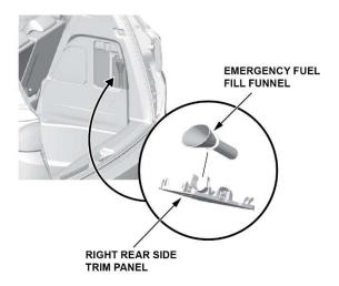
2. Insert the emergency fuel fill funnel into the fuel filler neck to relieve the pressure in the fuel tank.
