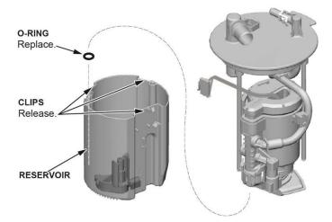
31. Release the three clips at the base of the fuel pump assembly and remove it from the fuel filter.
