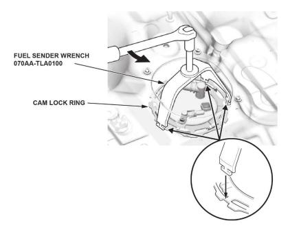
18. Turn the fuel tank unit cam lock ring counterclockwise to unlock it.
