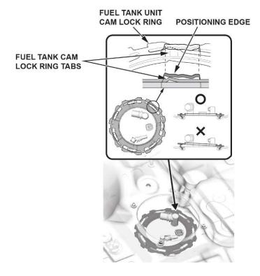
47. Tighten the fuel tank unit cam lock ring by turning clockwise using the fuel sender wrench.
