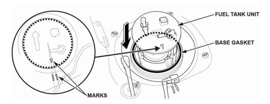
38. While pushing down on the fuel tank unit, make sure the fuel tank unit is flat against the base gasket. To avoid a leak and/or damaging the gasket, make sure the gasket is not pinched. Do this either visually and/or by hand.
