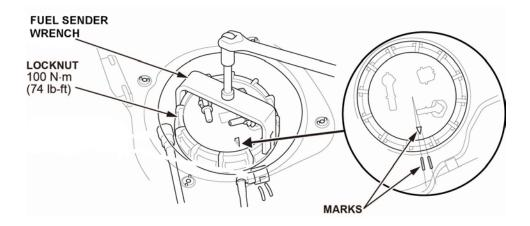
44. *If the marks do not line up*, friction between the fuel tank unit and the locknut may cause the fuel tank unit to turn while tightening. Observe the difference (shaded area), and loosen the locknut until the fuel tank unit can be rotated. Rotate the fuel tank unit **counter-clockwise** by the same amount, and repeat the tightening process.
