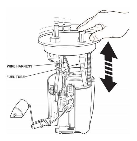
34. Clean the seal surfaces on the fuel tank unit and gasket groove on the fuel tank.
