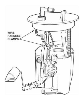
18. Press the tab on the fuel level sensor to release the lock. Then, push up on the fuel level sensor.
