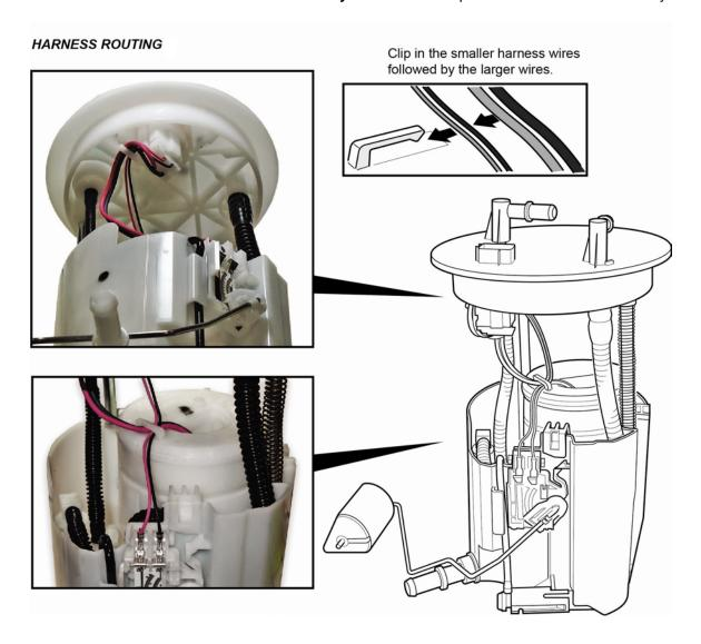
33. While compressing the fuel tank unit, make sure the movement is smooth and the fuel tube and wiring harness do not stretch, pinch, or bind.
