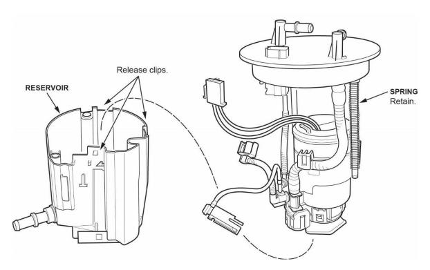
24. Release the three clips at the base of the fuel pump assembly and remove it from the fuel filter.
