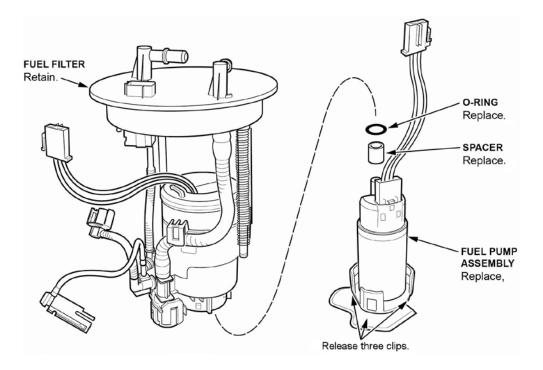
25. Pull the fuel pump assembly out of the fuel filter.
