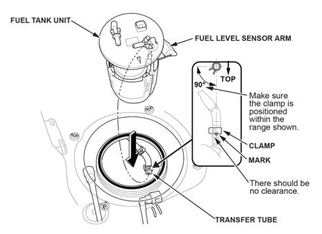
37. Line up the mark on the fuel tank unit to the marks on the fuel tank, then insert the fuel tank unit into the fuel tank. NOTE: To avoid any leaks, check the O-ring, either visually or by hand, to make sure it is not pinched.
