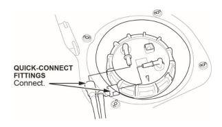
47. Connect the fuel tank unit connector.
