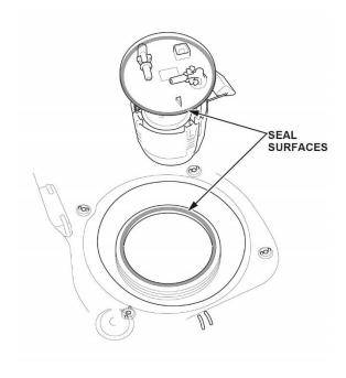
35. Carefully install a new base gasket to the gasket groove on the fuel tank as shown.
