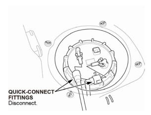
14. Loosen the fuel tank unit locknut using the Fuel Sender Wrench (T/N 070AA-T0AA100 or 07AAA-T0AA100), then remove it.
