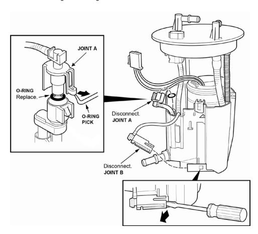
22. Disconnect joint B from the bottom of the reservoir.
