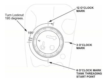
42. To keep the fuel tank unit parallel to the opening in the fuel tank, push down at the 3 o'clock mark while turning the locknut clockwise by hand.
