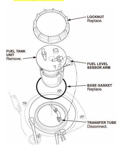
16. Prepare the fuel pump and parts to be replaced.
