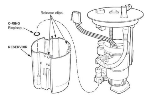
25. Release the three clips at the base of the fuel pump assembly and remove it from the fuel filter.
