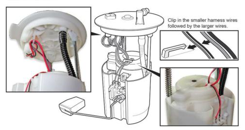
33. While compressing the fuel tank unit, make sure the movement is smooth and the fuel tube and wiring harness do not stretch, pinch, or bind.
