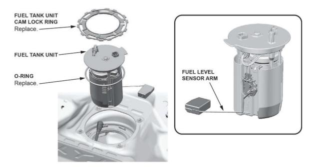
19. Prepare the fuel pump and parts to be replaced.
