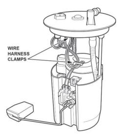
21. Press the tab on the fuel level sensor to release the lock. Then, push up on the fuel level sensor.
