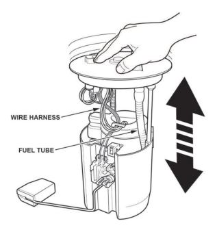
34. Install the fuel tank unit into the fuel tank with a new O-ring.
