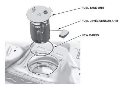
35. Line up the tab of the fuel tank unit as shown, and partially install the new fuel tank unit cam lock ring with a new O-ring.
