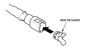
39. Connect the fuel line quick-connect fitting.
