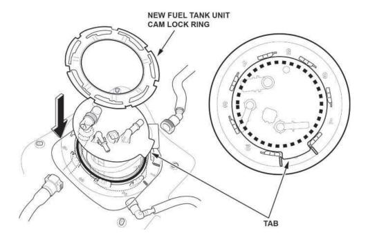
55. Connect the fuel vent tube and fuel tank vapor recirculation tube by slightly turning the fuel tank unit counterclockwise.
