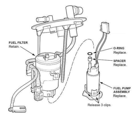
42. Install the new spacer, O-ring, and wire harness to the new fuel pump.
