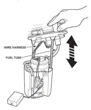
49. Install a new O-ring on the fuel tank.
