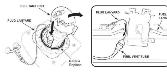
33. Remove the fuel tank unit with the O-ring.
