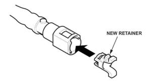
59. Connect the fuel line quick-connect fitting and connector.
