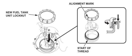
35. Press down on the fuel tank unit while turning the locknut clockwise by hand.
