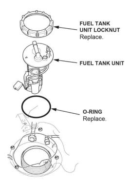
16. Prepare the fuel pump and parts to be replaced.
