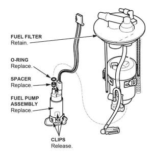
24. Pull the fuel pump assembly out of the fuel filter.
