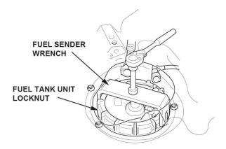
15. Remove the fuel tank unit.
