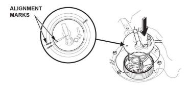
34. Line up the mark on the new locknut to the start of the thread on the fuel tank.
