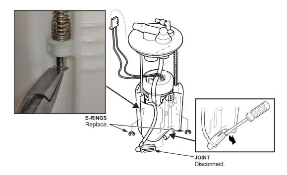
21. Disconnect the joint at the bottom of the reservoir.
