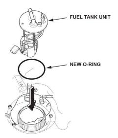
33. Line up the mark on the fuel tank unit to the marks on the fuel tank, then insert the fuel tank unit into the fuel tank. NOTE: To avoid any leaks, check the O-ring, either visually or by hand, to make sure it is not pinched.
