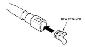
38. Connect the fuel line quick-connect fitting.
