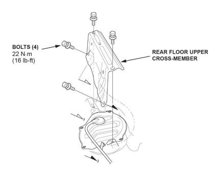
12. Remove the fuel tank unit access panel and disconnect the connector.
