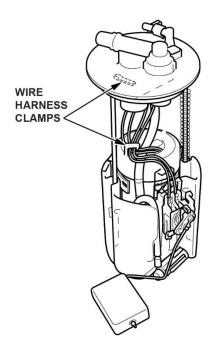
18. Press the tab on the fuel level sensor to release the lock. Then, push up on the fuel level sensor.
