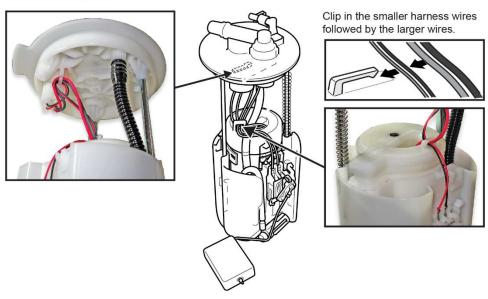
31. While compressing the fuel tank unit, make sure the movement is smooth and the fuel tube and wiring harness do not stretch, pinch, or bind.
