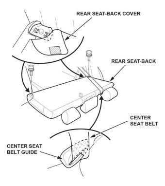
8. Pull out the center seat belt through the center seat belt guide, and remove the rear seat-back.
