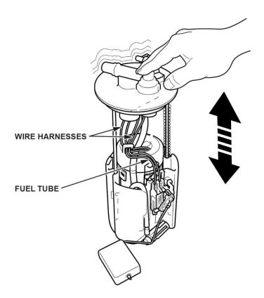
32. Install the new O-ring to the fuel tank, then partially install the new fuel tank unit.
