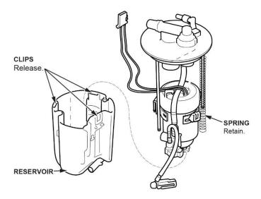
23. Release the three clips at the base of the fuel pump assembly and remove it from the fuel filter.
