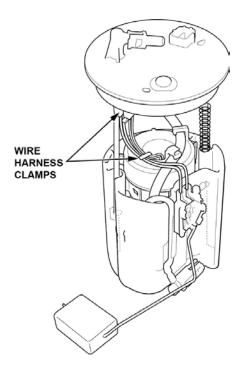
23. Press the tab on the fuel level sensor to release the lock. Then, push up on the fuel level sensor.
