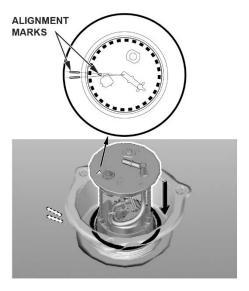
40. Line up the mark on the new locknut to the start of the thread on the fuel tank.
