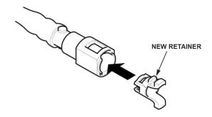
45. Connect the fuel line quick-connect fitting.
