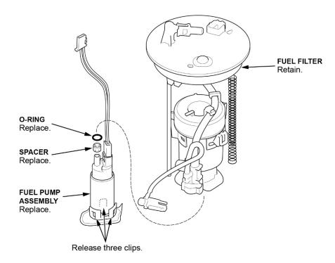
28. Pull the fuel pump assembly out of the fuel filter.
