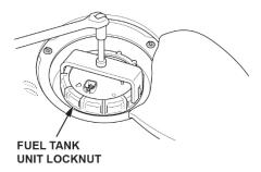
20. Remove the fuel tank unit locknut, then remove the fuel tank unit.
