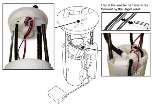
37. While compressing the fuel tank unit, make sure the movement is smooth and the fuel tube and wiring harness do not stretch, pinch, or bind.
