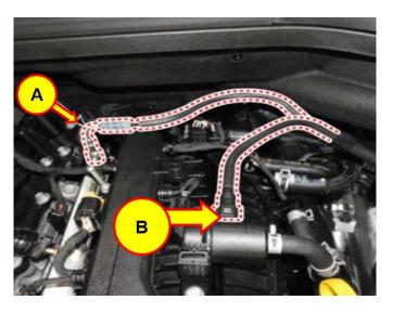
3. Disconnect the engine wiring connector and harness fasteners of the intake manifold.
