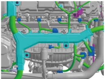
4. Then remove the engine upper connectors & wiring.
