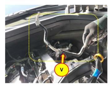
21. Install the supplied pipe and reinstall the removed parts in reverse order of removal.
