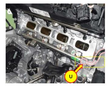
20. Remove and discard the high-pressure fuel pipe (V).
