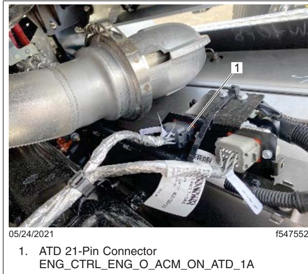
Fig. 12, ATD 21-Pin Connector ENG_CTRL_ENG_O_ACM_ON_ATD_1A Location
