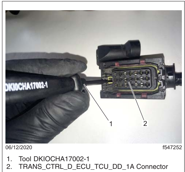
Fig. 3, Releasing the 21-Pin Connector Secondary Lock
