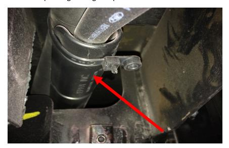
Step 8- Lift tank back into place and tighten down tank. Torque to 52ft/lbs.
