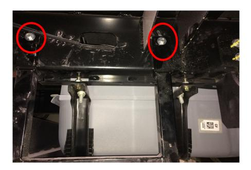
Step 3- Loosen all four bolts (2 per side) that hold the gas tank to the frame. Use the 17mm wrench and 5/8" socket. NOTE: Do not completely remove bolts or drop gas tank out.
