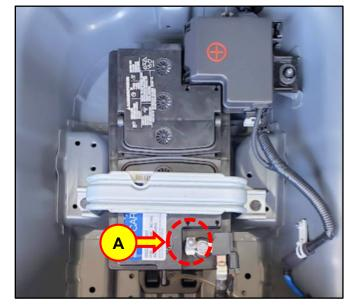
3. Open the hood and remove the engine room fuse box upper cover and discard.
