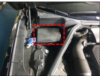
4. Remove the ESC/VDC1, ESC/VDC2 40A fuses (B).
